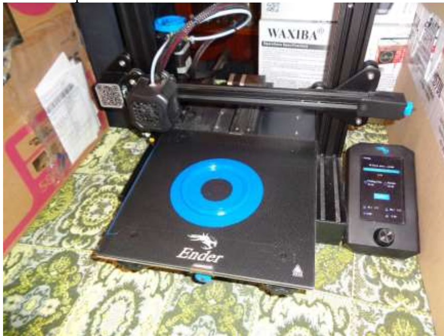
Figure 7. "Press Bushing" landmark, 3D printed using ABS+ filament on Creality 3D printer, Ender 3 V2
