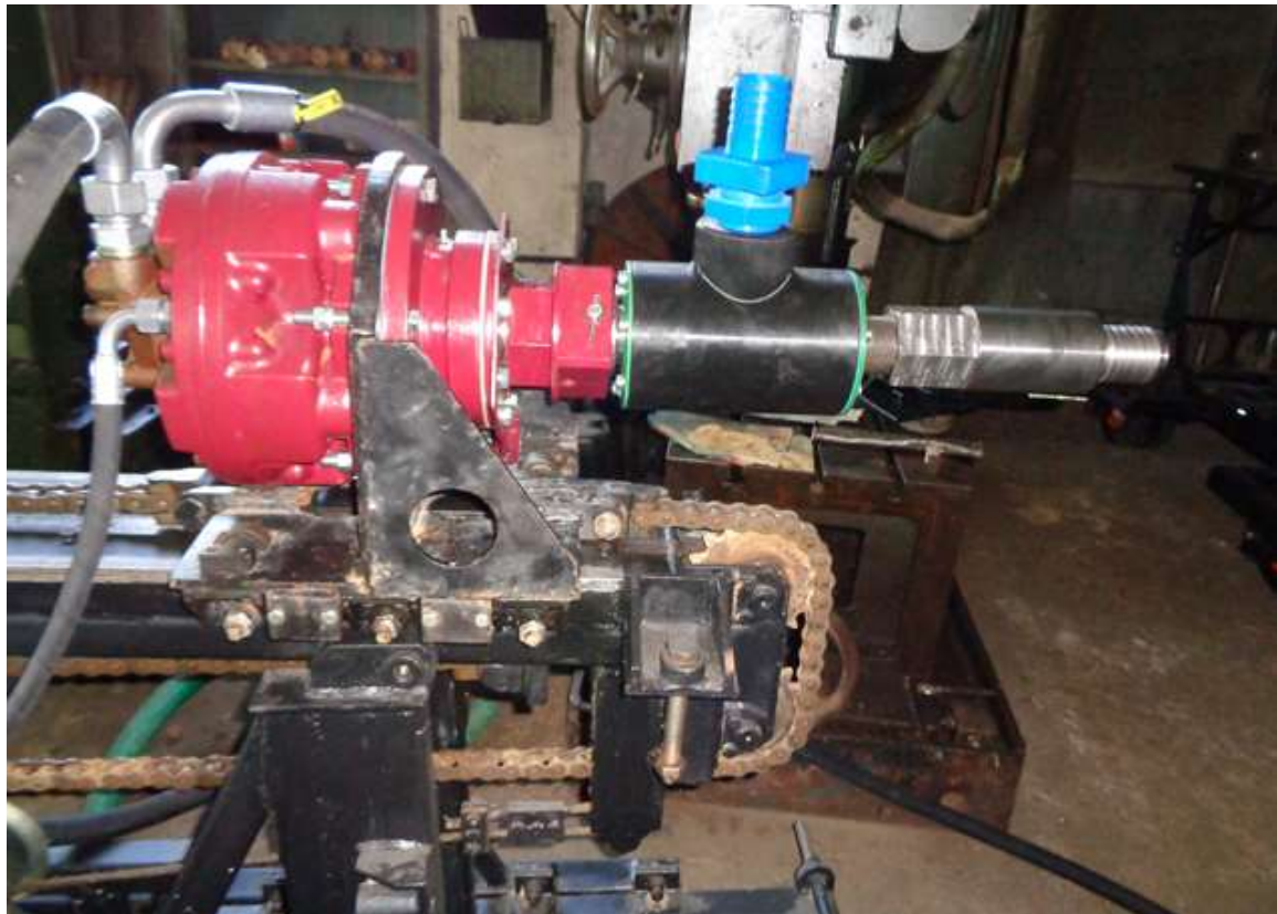
Figure 8 Integration of 3D printed landmarks to the FA 125-FG 40 drilling rig
