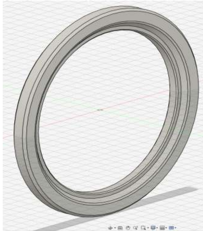
Figure 3. 3D modeling in the Autodesk Fusion 360 program of the "Press Bushing" part, resulting in the STL format file for "slicing" before its 3D printing
