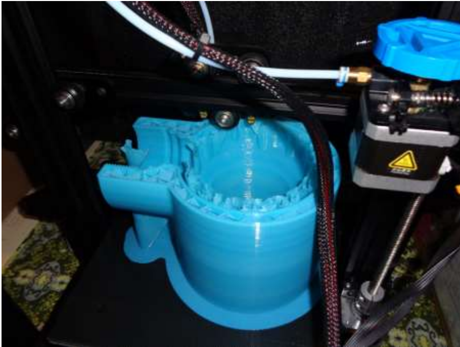
Figure 5. 3D printing of the FA 100 washing head housing
