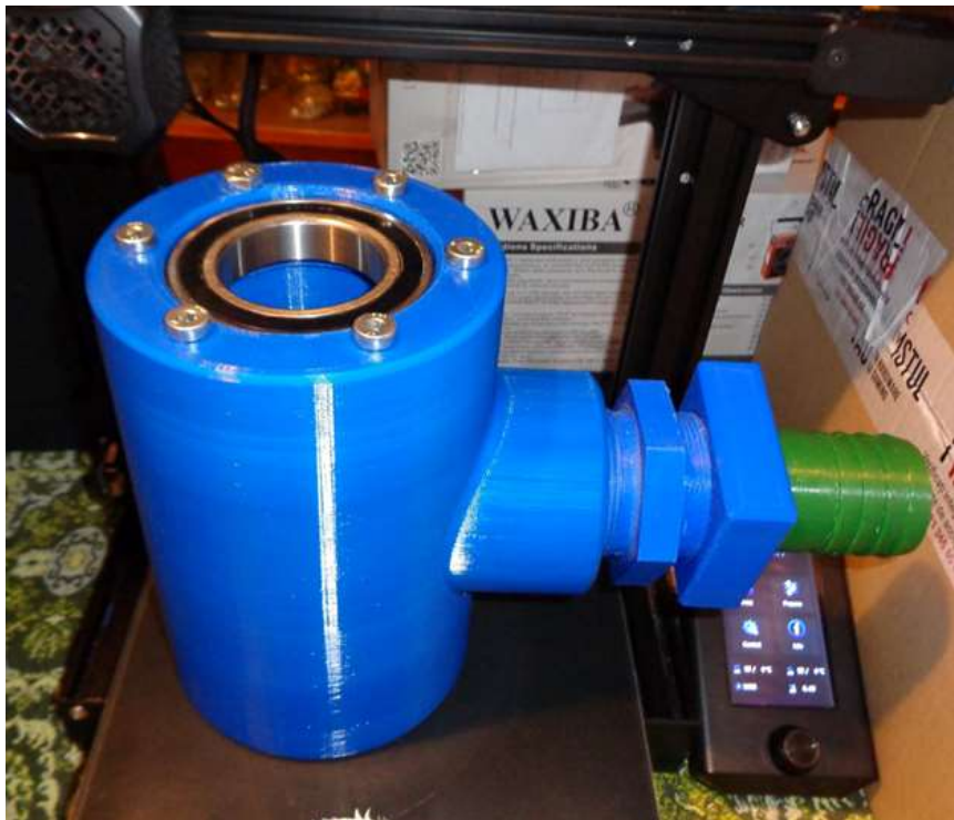
Figure 6. 3D printed washing head housing
