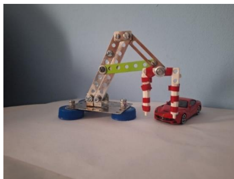
Fig. 3 The barrier mechanism for access to the parking lot provided with the access frame in the lower position (mockup, own contribution)
