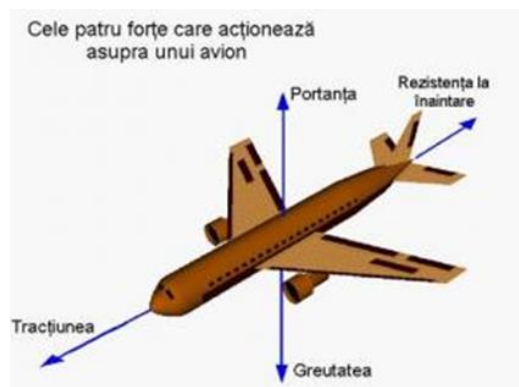
Figure1. The four forces acting on an airplane. [3]
