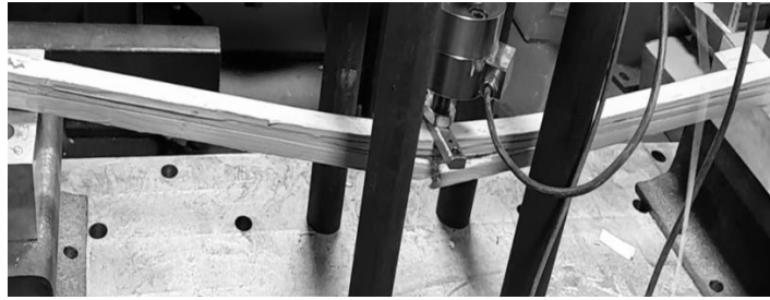
Fig.6 Pine slats package consolidated with epoxy resin, tested in bending
