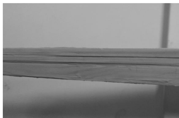
Fig.5 Pine slats package consolidated with epoxy resin
