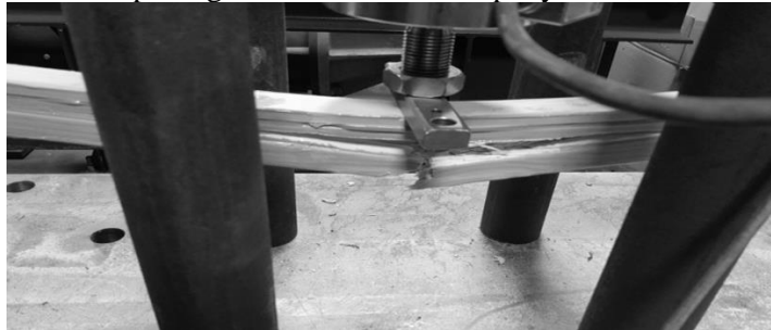
Fig.7 Fracture detail for pine slats package consolidated with epoxy resin
