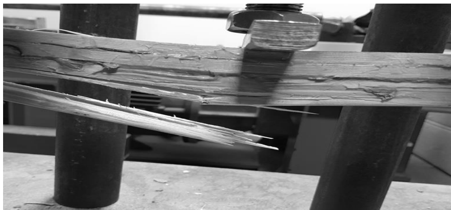
Fig.10. Fracture detail for pine slats package consolidated with carbon fiber fabric and epoxy resin
