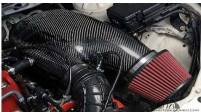
Figura 1. Tuning filtru de aer conic Figure1. Conical air filters for engine tuning
