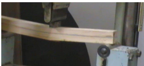
Figura 1. Grinzi ranforsate cu CFRP [6] Figure 1. CFRP sheet reinforced wood beams (6)
