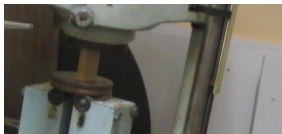
Figura 2 a). Stâlp neranforsat [6] Figure 2 a). Un-reinforced wood column [6]
