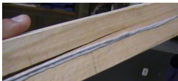
Figura 1. Grinzi ranforsate cu CFRP [6] Figure 1. CFRP sheet reinforced wood beams (6)
