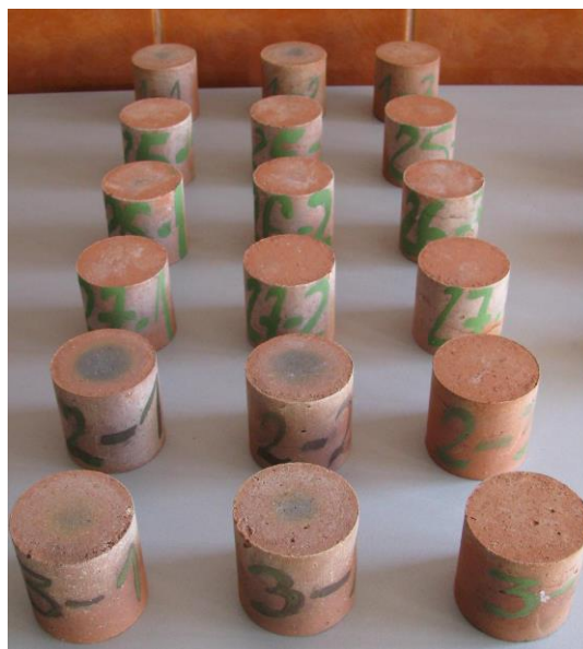
Figure 2. Set of cylindrical specimens heat treated
