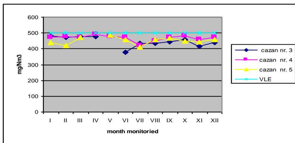
Fig.2. The evolution of NO<sub>2</sub> concentration in the flue gases in 2011
