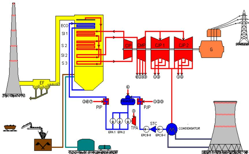
Fig. 1. Schematic diagram of power generation of 330 MW in the energy group
