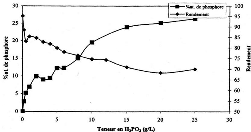
Figure 1. Influence of phosphorous acid in the electrolyte concentration on the phosphorus content in the layer and on the cathode performance [5]
