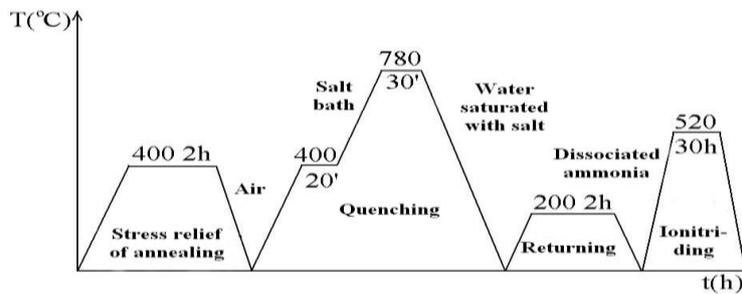
Fig.5 The heat treatment cycle of punches from OSC10 ionitriding
