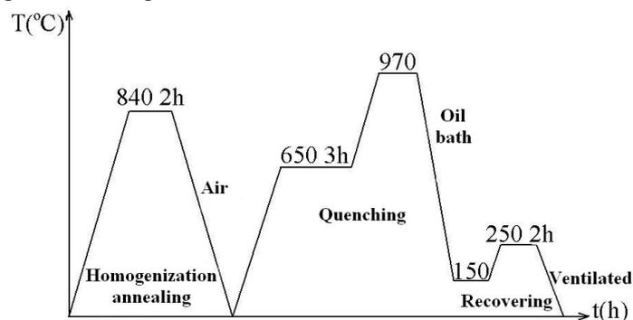
Fig.1 The heat treatment cycle of punches from 205Cr115
