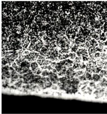
Fig.6 The structure of OSC10 ionitriding x200
