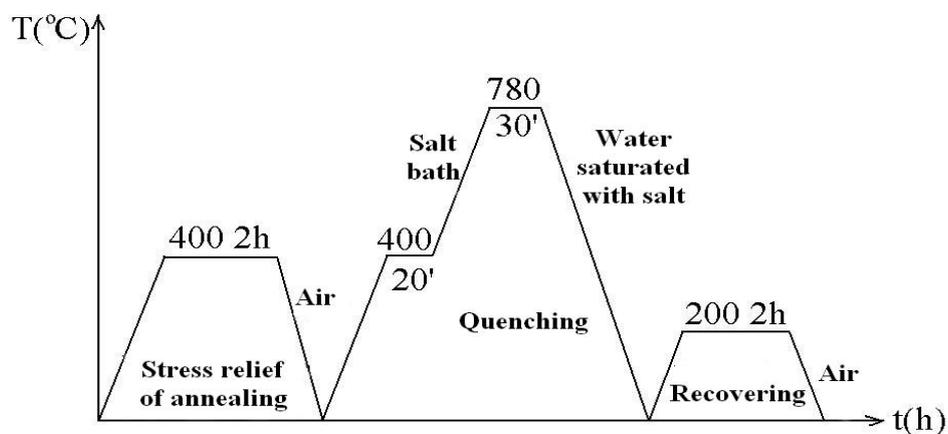
Fig.3 The heat treatment cycle of punches from OSC10
