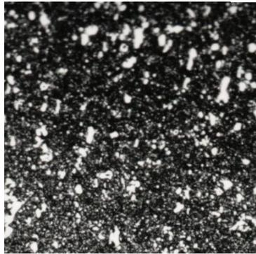
Fig.2 The structure of 205Cr115 hardened and tempered x400
