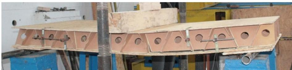
Figure 8. Strain at the breaking point for perpendicular to the faces of the panels load
