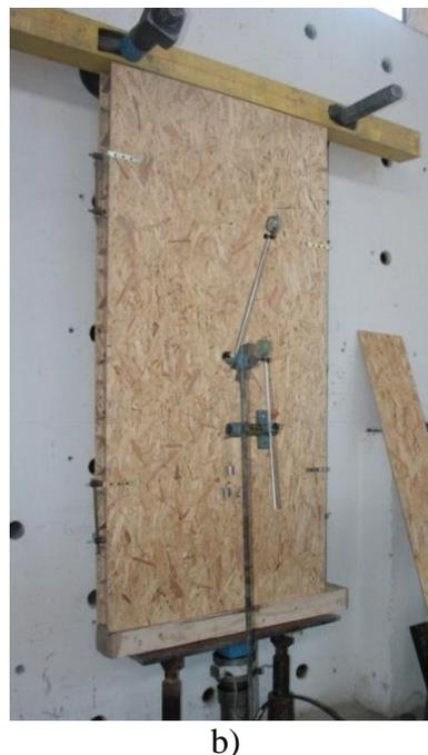
Figure 3. The stand with parallel load to the face of the panel. a) Scheme b) The testing stand
