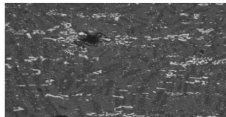
Fig.10. Core **1.2379CVNC** after nitrocarburated at 540 °C, 500:1
