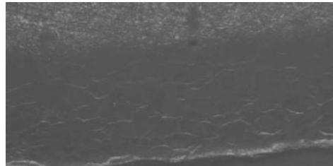
Fig.8. Coating **1.2343CVNC** nitrocarburated at 540 °C, surface hardness 1120 HV1 500: 1 ;
