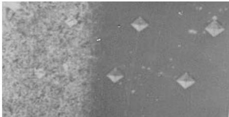
Fig.7. Coating **1.2343CVNI ionic** nitridated at 520 °C, surface hardness 1281 HV1 ; 500 : 1 white coating 5-10 microns,
