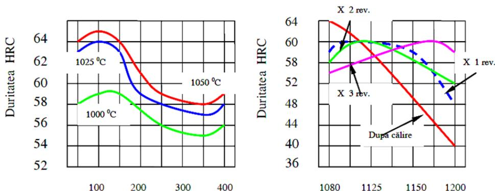
Fig 1.. The hardness of the alloyed steel 12, 5% Cr și 0,8 % V depending on the hardening temperature, respectively of the reversible temperature: a – reverse transformation at 100 – 400 0C ; b – repeated reversible transformation at 520 0C [5]
