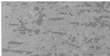
Fig.9. Core **1.2379CVNI** after ionic nitridation at 520 °C, 500:1
