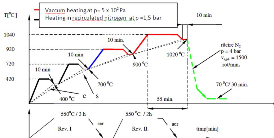
Fig.3. A Variant of thermic treatment previously applied to the nitridation in plasma / nitrocarburation
