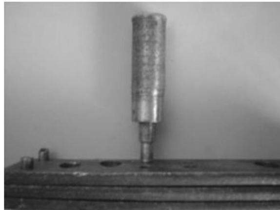
Fig.2. Punching drift for the semi manufactured spring sheets
