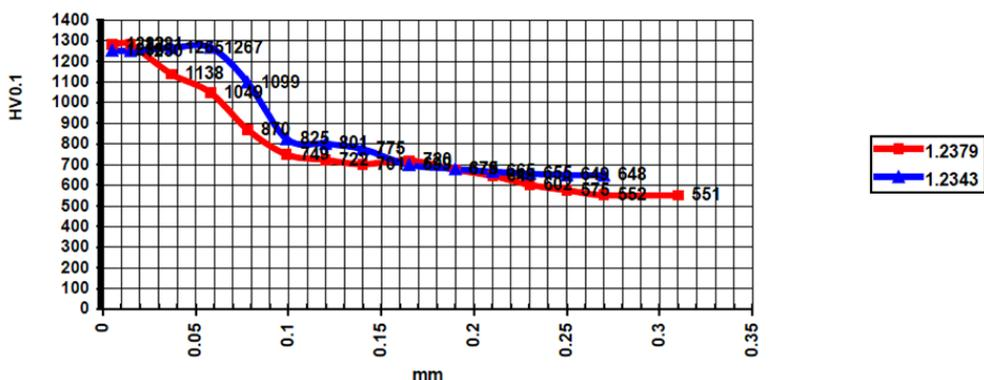
Fig.4. Variation of the microhardness for the steels W1.2343 si W1.2379, nitrided in plasma at 520° C
