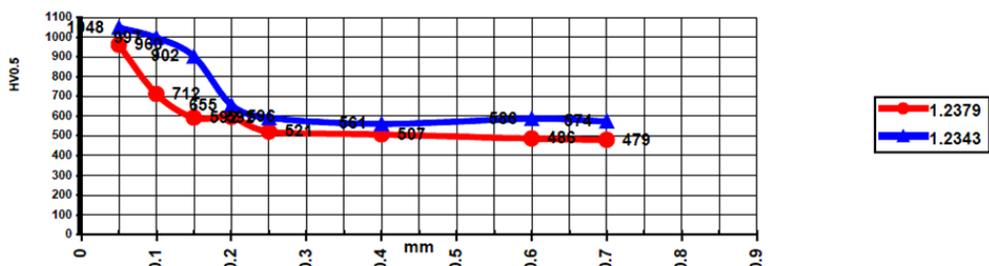
Fig.5. Variation of the microhardness for the steels 1.2343 and 1.2379, nitrocarburated at 540° C.
