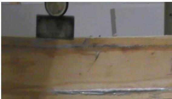
Fig. 3. Up and down reinforcement application: two sheets of composite material
