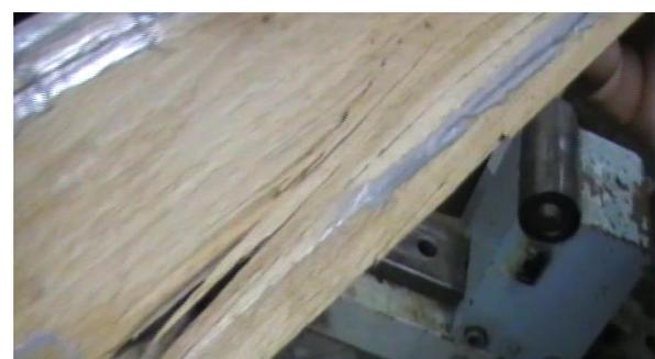
The wood beam samples were reinforced with Megaplate composite plates and carbon fiber sheets and bending subjected. All beams were surveyed for both their geometric dimensions and wood defects. The average value of the wood humidity ratio was 12%, while that of the wood density was  $449,6 \text{ kg/m}^3$ . The CFRP
