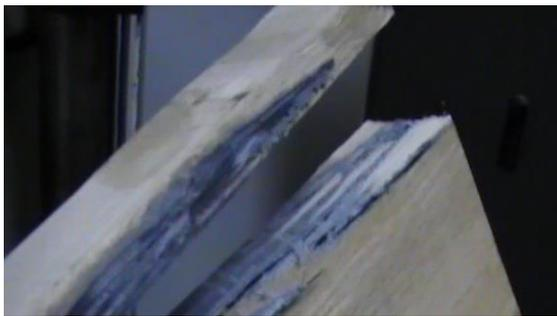
Fig. 2. Middle reinforcement application: one sheet of composite material
