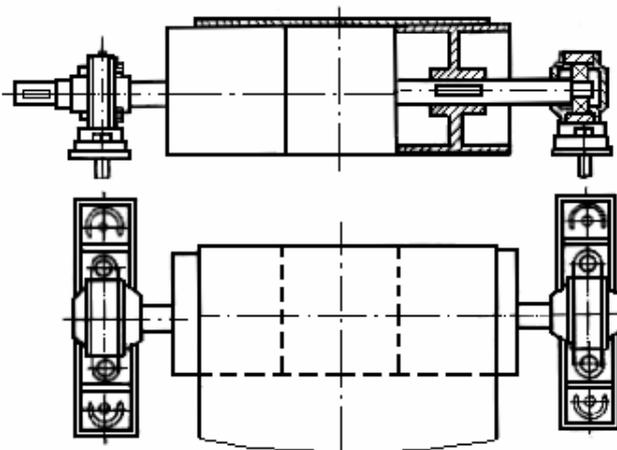
Figure 7. Mounting of a driven drum
