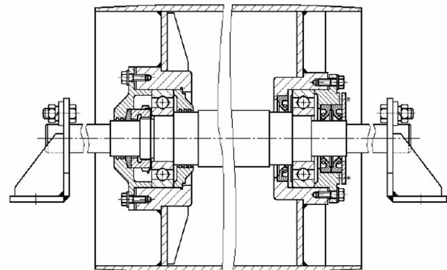
Figure 8. Mounting of a free drum
