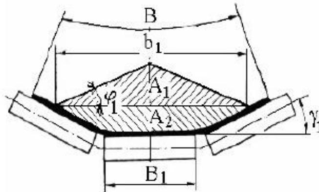
Figure 5. Section area trough material and belt
