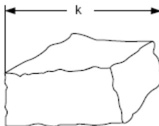
Figure 4. Dimension K for transported material
