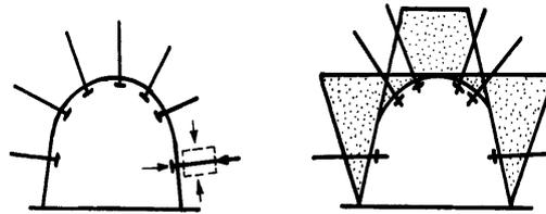
Fig. 4 Influence of anchored support to the development of more consolidation forces on the excavation contour
