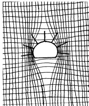
Fig. 5 Redistribution and centralization of tensions into the walls of the mining work
