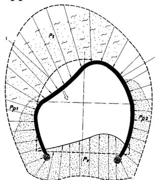
Fig.2. Non-uniform deformation mode of mining works performed with steel timbering, in the case of taking-over the maximum force from the wall located in front of the layer: 1- initial profile; 2- outcome profile after force stabilization
