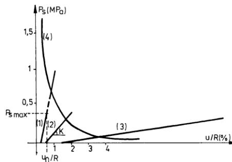
Fig.7 The role of consolidation in the interaction of "support – rock":  $U_0$  - rock deformation of around the underground excavation;  $R$  - radius of the mining work
