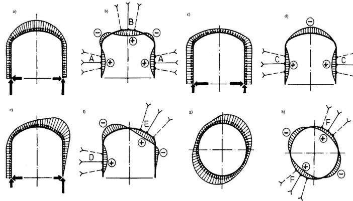
Fig. 6 The areas of maximum bending moments surrounding the underground excavations for different types of profiles and forces: a, b – the case of arch profile and maximum forces from the ceiling; c, d – the case of arch profile and maximum forces from the walls; e, f – the case of arch profile and maximum asymmetrical forces from the ceiling; g, h – the case of circular profile and maximum vertical forces (ceiling and floor)
