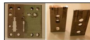
Figure 8. New shape of matrix and mandrels.
