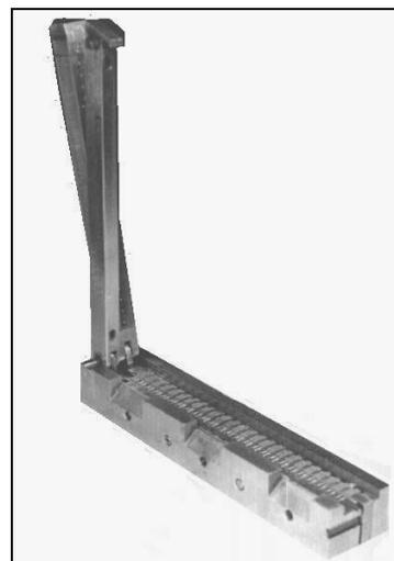
Figure 11. Device to inject the insulating mass.
