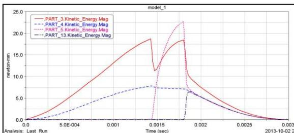
Figure 7. Kinetic energy of the pressing chain elements over the brass tape.
