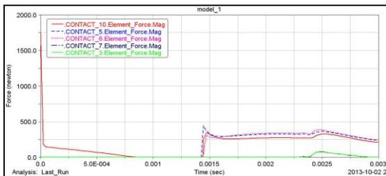
Figure 6. Variation of the contact forces from pressing chain couplings over the brass tape
