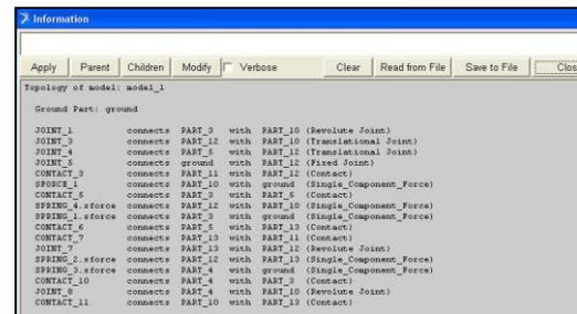
Figure 4. The connections between different elements of the model and exterior loads.
