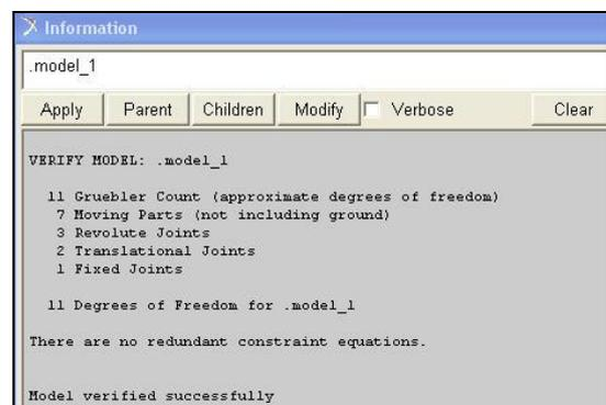
Figure 5. The verification result of the created model
