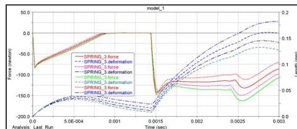
Figure 8. Variation of the reaction force and deformation of spring 8 for different values of the  $K$  stiffness coefficient.
