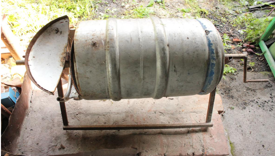
Fig.3. Assembly shown generally barrel is observed, load capacity, rotating crank goat metal barrel support
