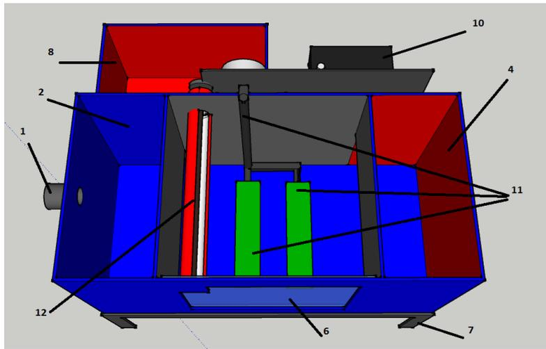
Figure 1 Scheme of construction of separator systems bubbling fats
