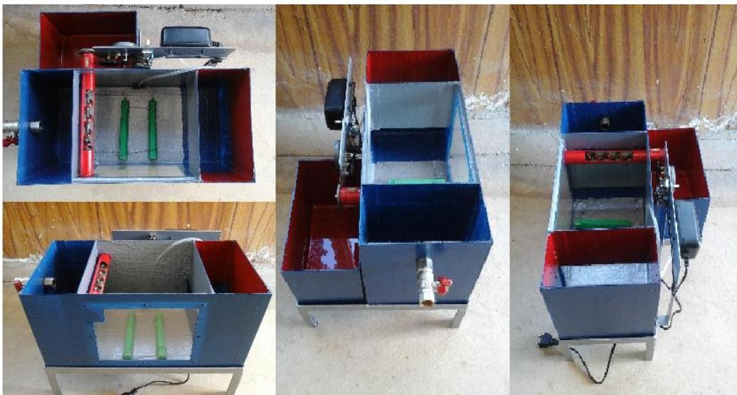
Figure 2. Grease separator
