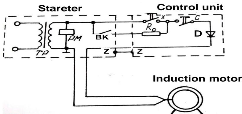
Fig. 1. Schematic diagram for automatic grounding control of mobile machines with remotely controlled induction motor
