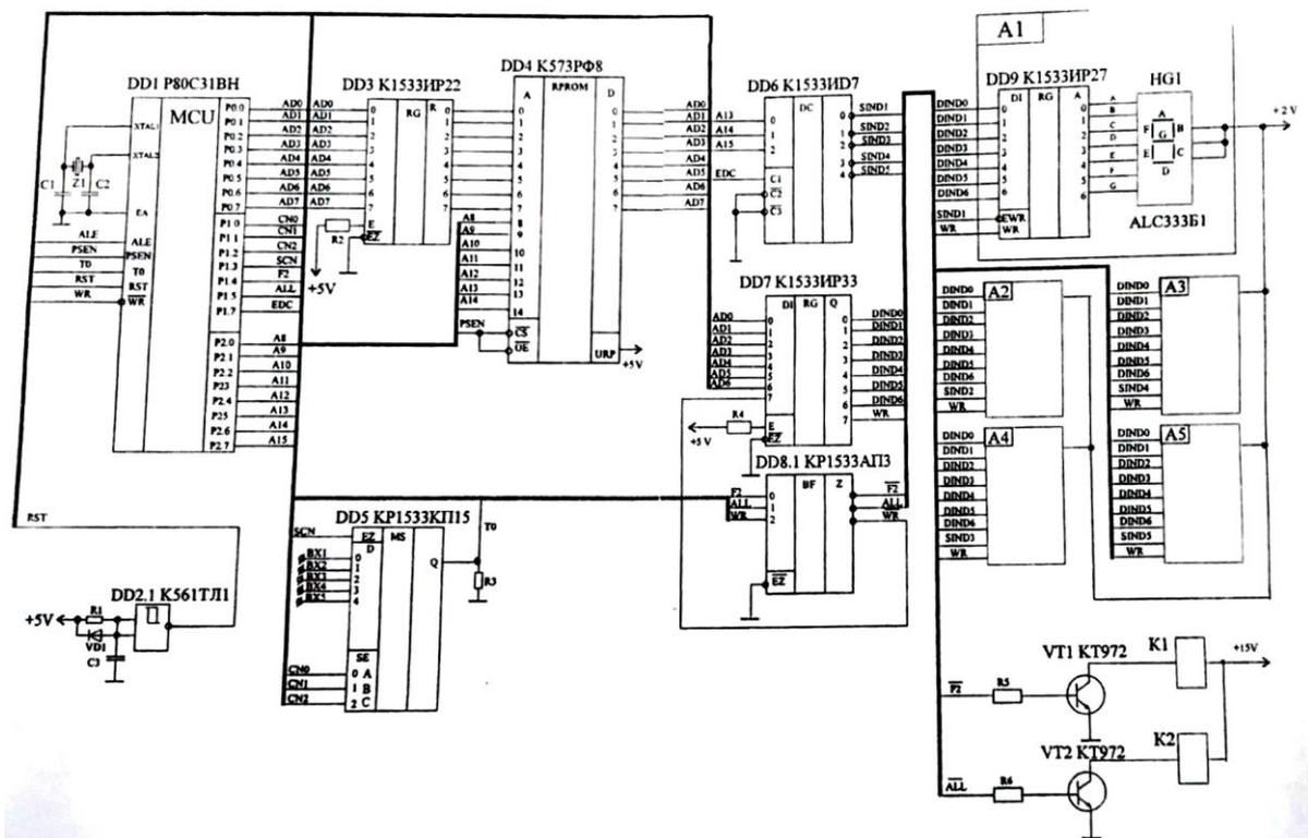
Fig. 5. Wiring diagram of unit for remote control and diagnostics type BUD
