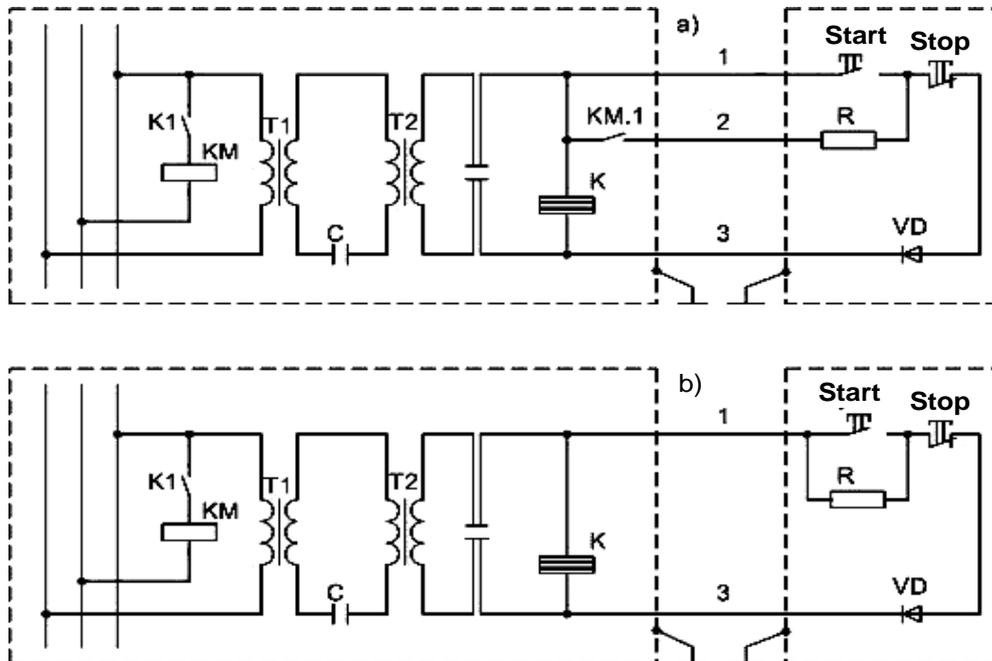
Fig.2. Three-wire (a) and two-wire (b) schemes for remote control of mobile machinery
