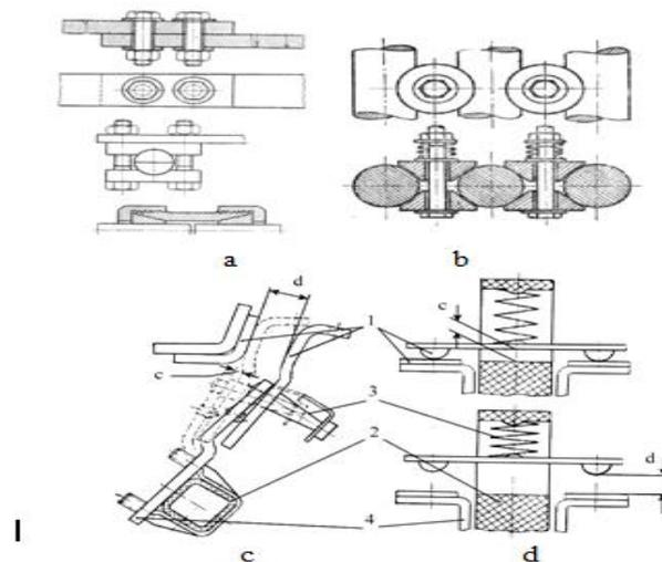
Figure1 Contact systems forms: a) with immovable contact ; b) with sliding contact; c) with a break contact; d)with two break contacts.
