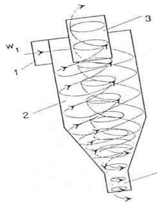
Fig.3. The function of a cyclone scheme: 1 - crude gas inlet; 2 - cylindrical housing; 3 - purified gas outlet tube; 4 - dust discharge tube
