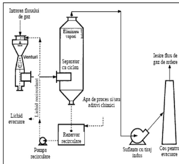
Fig. 4. Typical flow diagram of the system Venturi (Ciemat, 2000)
