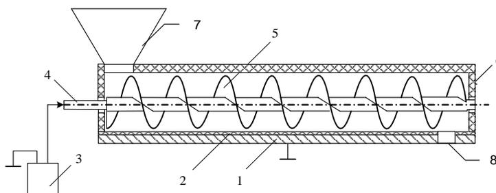
Fig. 1. Device for pre-sowing electromagnetic treatment of seed material: 1 – metal casing; 2 – dielectric coating; 3 – high voltage source; 4 – shaft; 5 – metal screw; 6 – insulation flanges; 7 – inlet opening; 8 – outlet opening
