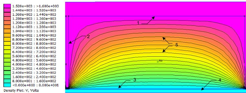
Fig.2a) Computer model of the equipotential lines of the electric field of the treatment device with no seeds in it:
