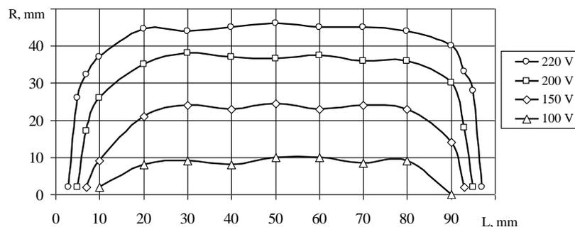
Fig. 2b) Results of the experimental study of the field [4] – equipotential lines
