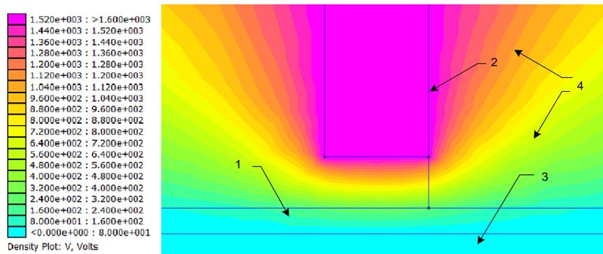
Fig. 3 Model of the equipotential lines of the electric field of the treatment device in the area below the vertex of the screw:
