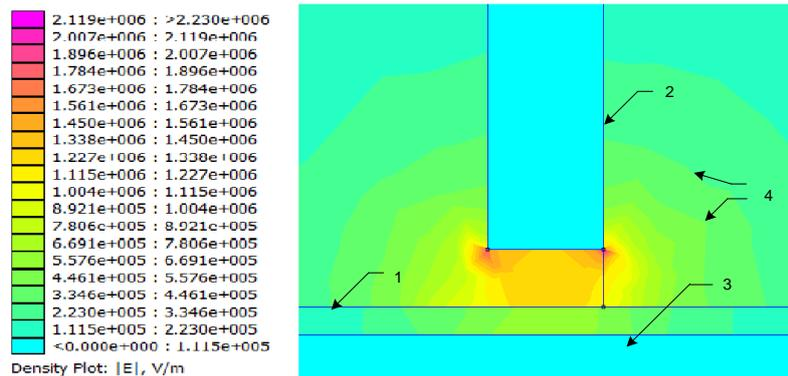
Fig.4 Model of the electric field strength in the area below the vertex of the thread: 1 –
