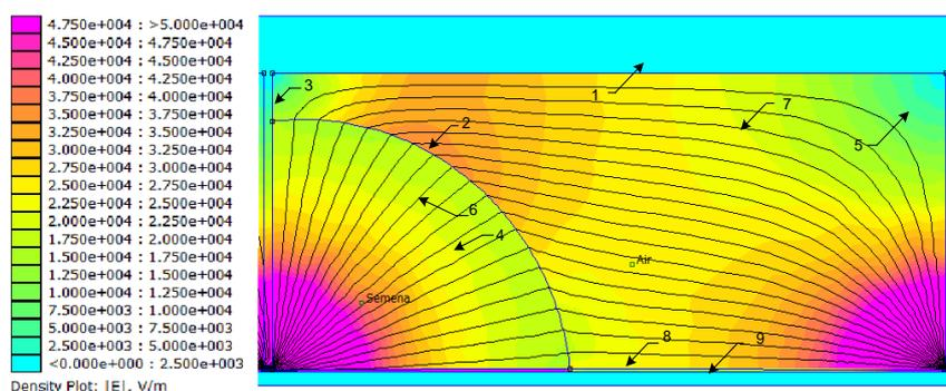
Fig. 1a) Computer model of the image of the field of the treatment device with seeds present (in the form of grain piles) in the inter-electrode space (the denotations 1 to 9 are explained under Fig. 1b).
