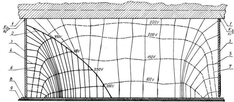
Fig. 1b) Experimentally obtained image of the electric field in the treatment device when full of seeds forming grain piles [3]:
