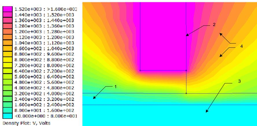
Fig. 2. Image of the electric field of the treatment device in the area below the thread, with seeds present in the device: 1 – Hostaphan; 2 – vertex of the screw; 3 – metal casing; 4 – equipotential lines
