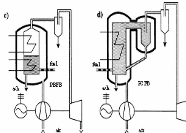
Figure 1. Fluidized bed combustion plants
