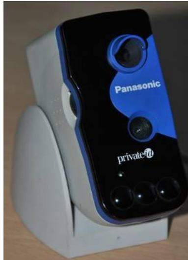
Figure 4. Panasonic BM-ET100US camera for iris and/or face recognition
