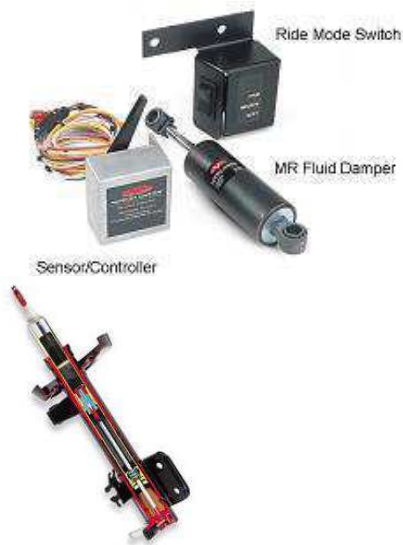
Fig. 2. Damper MR auto (operating)
