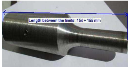
Figure 1. A practicably realized ultrasonic horn
