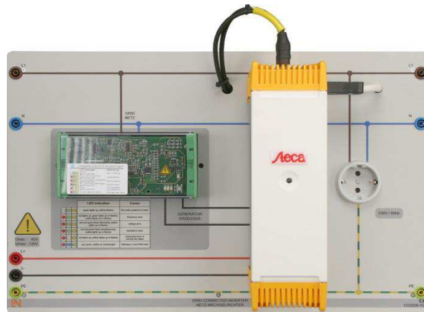
Fig.6. The ON-GRID inverter
