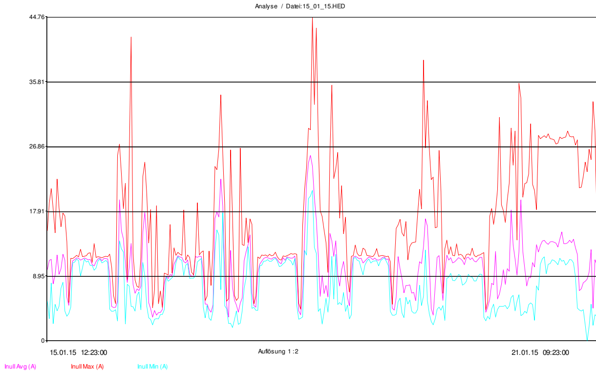
Figure 3. Minimum, maximum and average currents flowing through the transformer’s neutral, measured for intervals of 15 min. during the period 15.01.15 – 21.01.15
