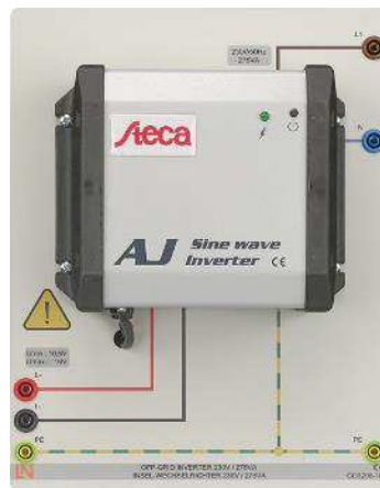
Fig.5. The OFF-GRID invertor
