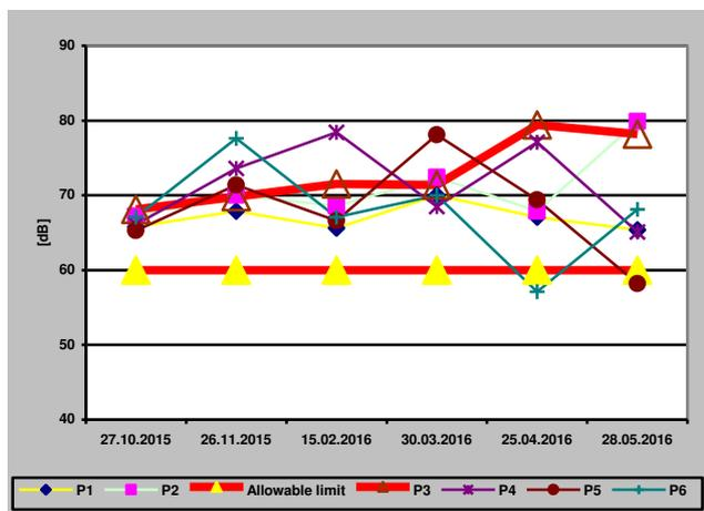
Fig. 4. The graphical representation of the results of monitoring noise level Leq
