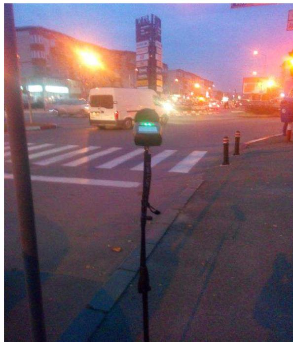
Fig. 2. Location sound meter according to SR ISO 1996-2: 2008
