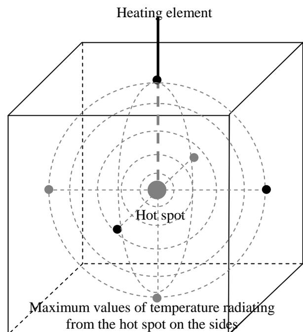
Figure 5 Heat conduction from hot spot towards the surface of the cube
