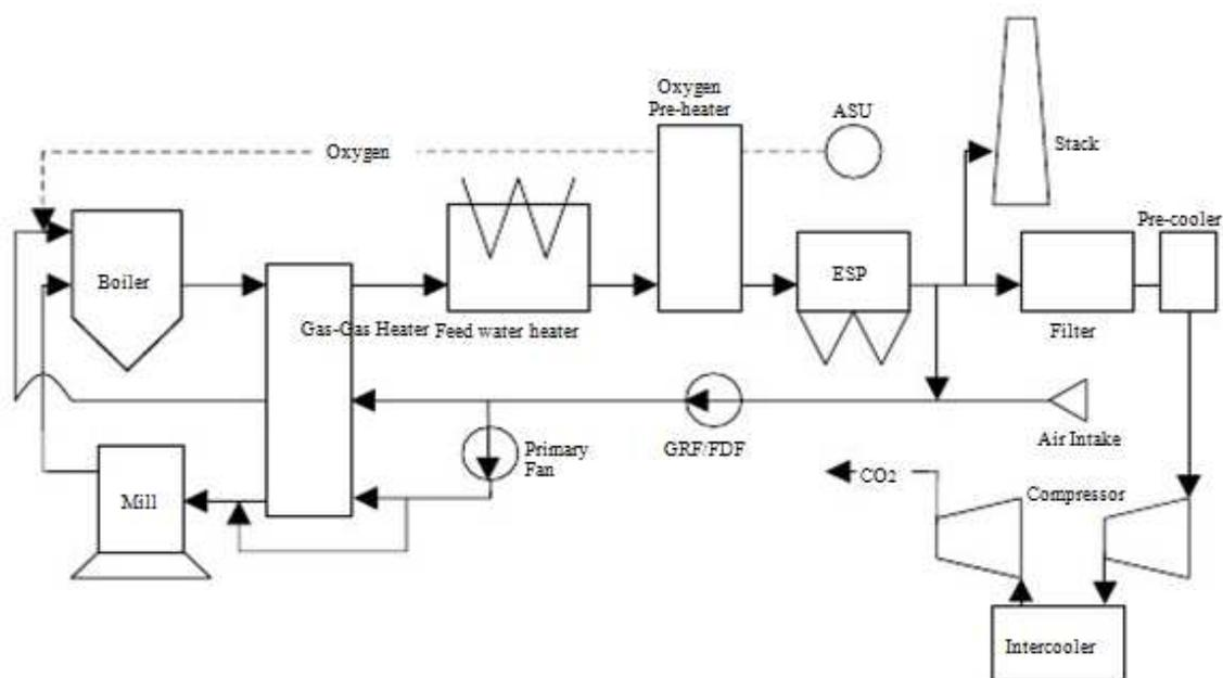
Figure 2. Pulverized coal-fired power plant using oxy firing combustion
