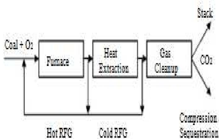
Figure 1. General flow sheet for oxy-fuel combustion
