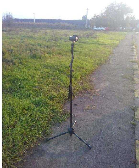
Fig. 2. Location sound meter according to SR ISO 1996-2: 2008
