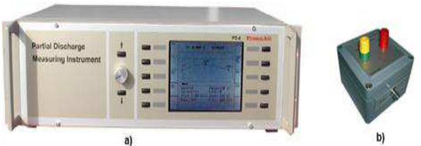
Figure 1. The measurement system of partial discharges
