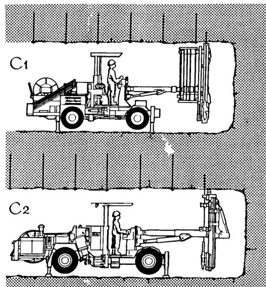
Figure 2. Installations used for fully mechanised mounting of anchors: **C<sub>1</sub>**-Installation for mounting Swellex anchors; **C<sub>2</sub>**-Installation for mounting different types of anchors.
