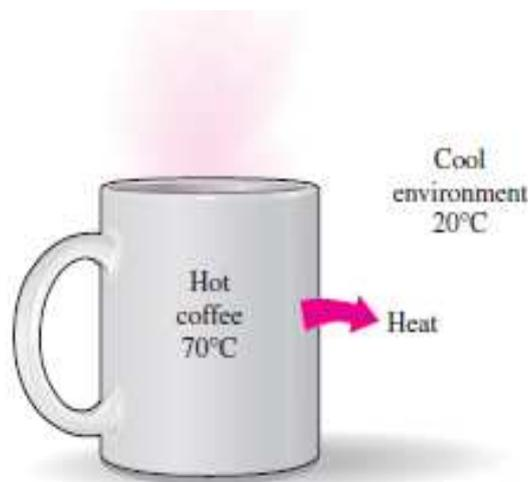
Figure 3 Heat flows in the direction of decreasing temperature
