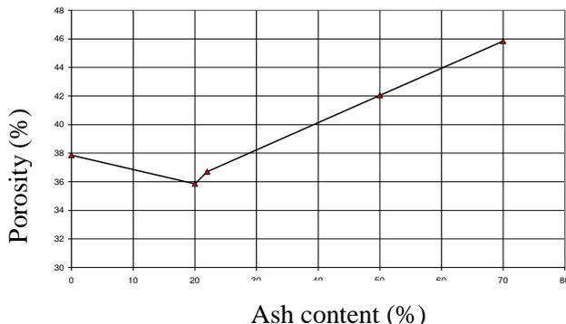
**Figure no. 3** Porosity dependency on the mixture ash content [7]
