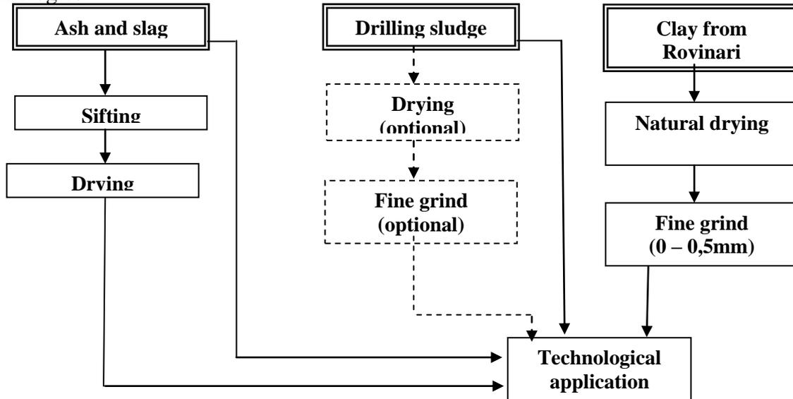
**Figure no 1.** The flowchart of the primary processing of waste flow
