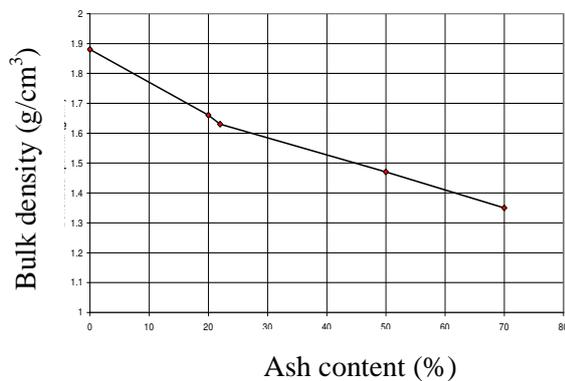
**Figure no. 2** Bulk density dependency on the mixture ash content [7]
