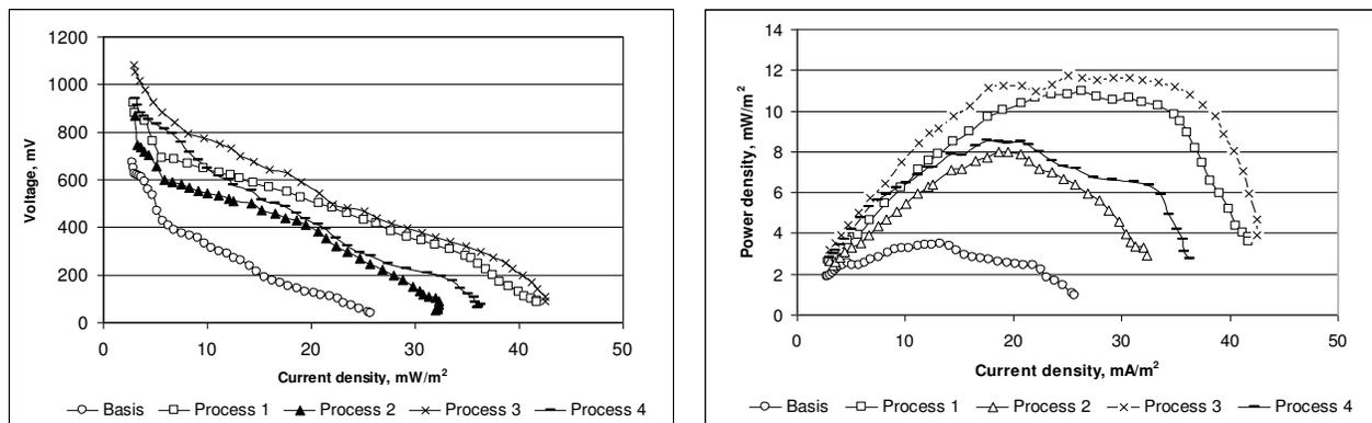
Figure. 2. Polarization curves of PSMFC`s
