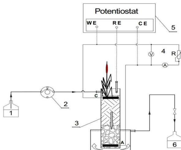
**Figure 1.** Design of Plant sediment microbial fuel cell
