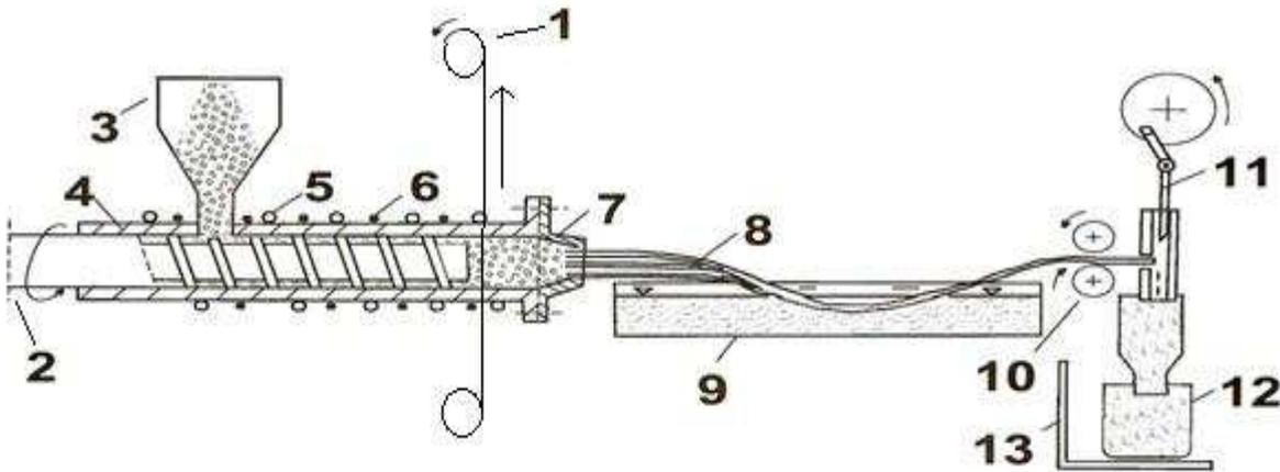
**Fig 2 . Schematic diagram of a plant for producing plastic pellets**
