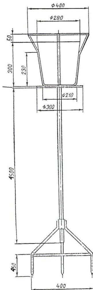
**Figure 2. The settled powders sampling device.**
