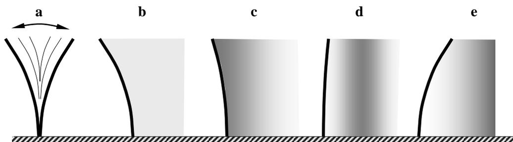
**Figure nr. 1.** Transmitting sonorous waves by air. a. the vibration of an elastic blade; b. c. d. e. compression and relaxation stages of the air.
