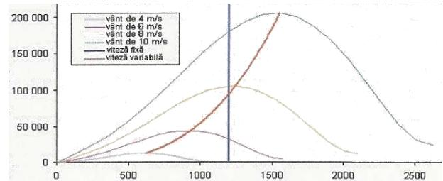
Power depending on the speed of rotation of the shaft
