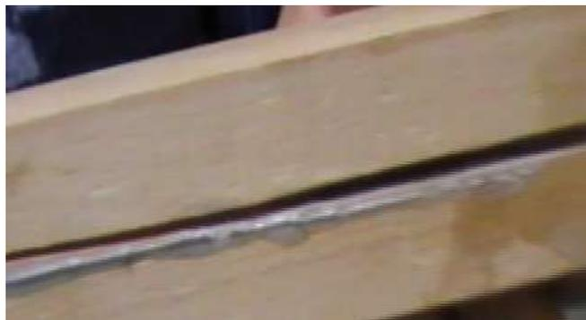
Fig. 2. Middle reinforcement application: one sheet of composite material [4]
