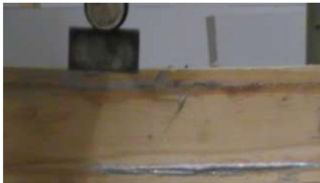
Fig. 3. Up and down reinforcement application: two sheets of composite material [4]
