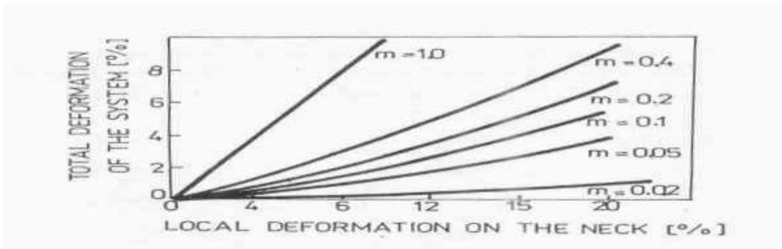
Fig.2 Relationship between the size of local deformation of necks and macrodeformation
