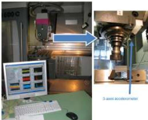
Fig. 4. Experimental log acceleration device to the shaft of the machine tool during the milling micromachining.
