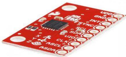
Fig. 2. -Accelerometer sensor designed to measure line throttle
