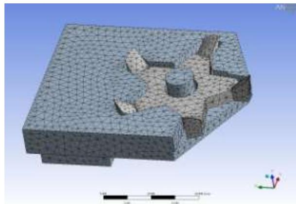
Fig. 4. Meshing the model stellate insert and its support
