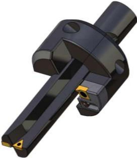
Fig. 2. Combined cutting tool - type Sandvik drill with chamfering modul with square insert with spout for chamfering, frontal located, fixed central with screw.
