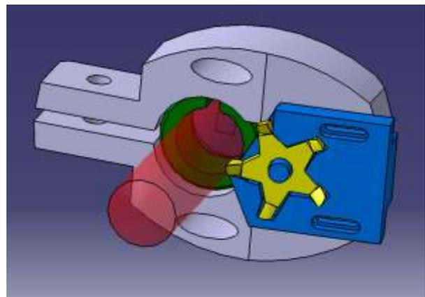
Fig. 1. Constructive tool solution for beveled and drill - with adjustable support with a special form of inserts (star-shaped).
