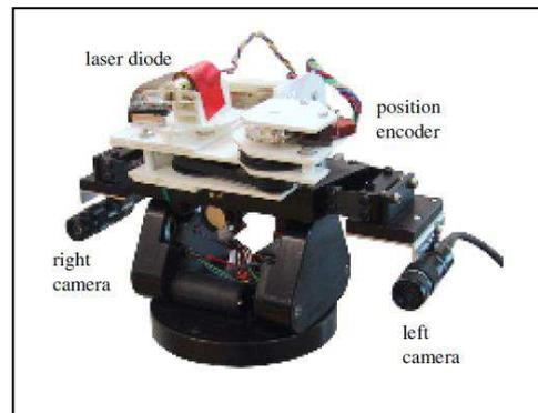
Fig. 6. Experimental stereoscopic light stripe scanner.
