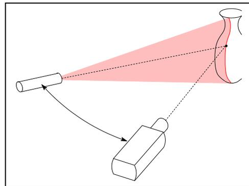
Fig. 1. Conventional single-camera light stripe sensor
