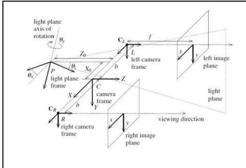
Fig. 4. Light stripe camera system model
