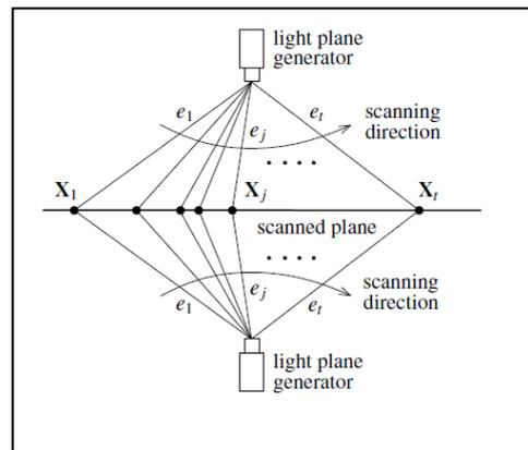
Fig. 5. Possible positions of the light plane from the scan of a planar calibration target. The position of the light plane generator is ambiguous.
